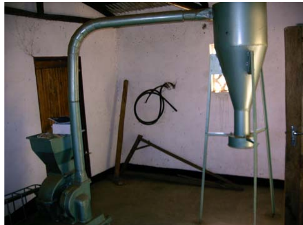
Maize mill project that has stayed since 2004 not being operated due to lack of electricity connection at Mpokonyola CBO – 30/05/2008
